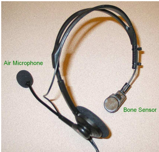
Figure 1: Air and bone sensors mounted on a headset
